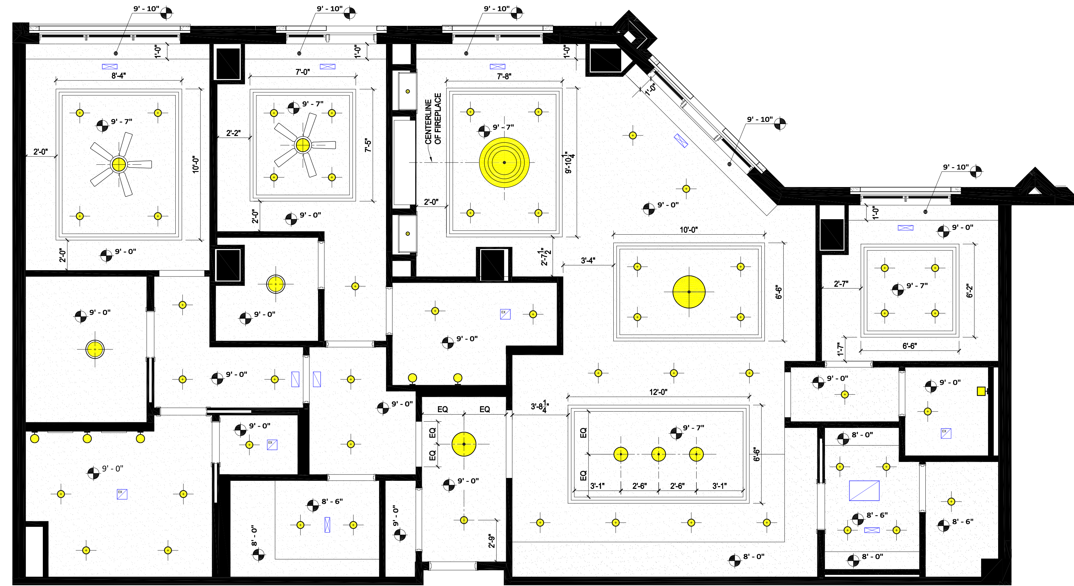
2 CONDO UNIT 103 - REFLECTED CEILING PLAN 1/4" = 1'-0"
