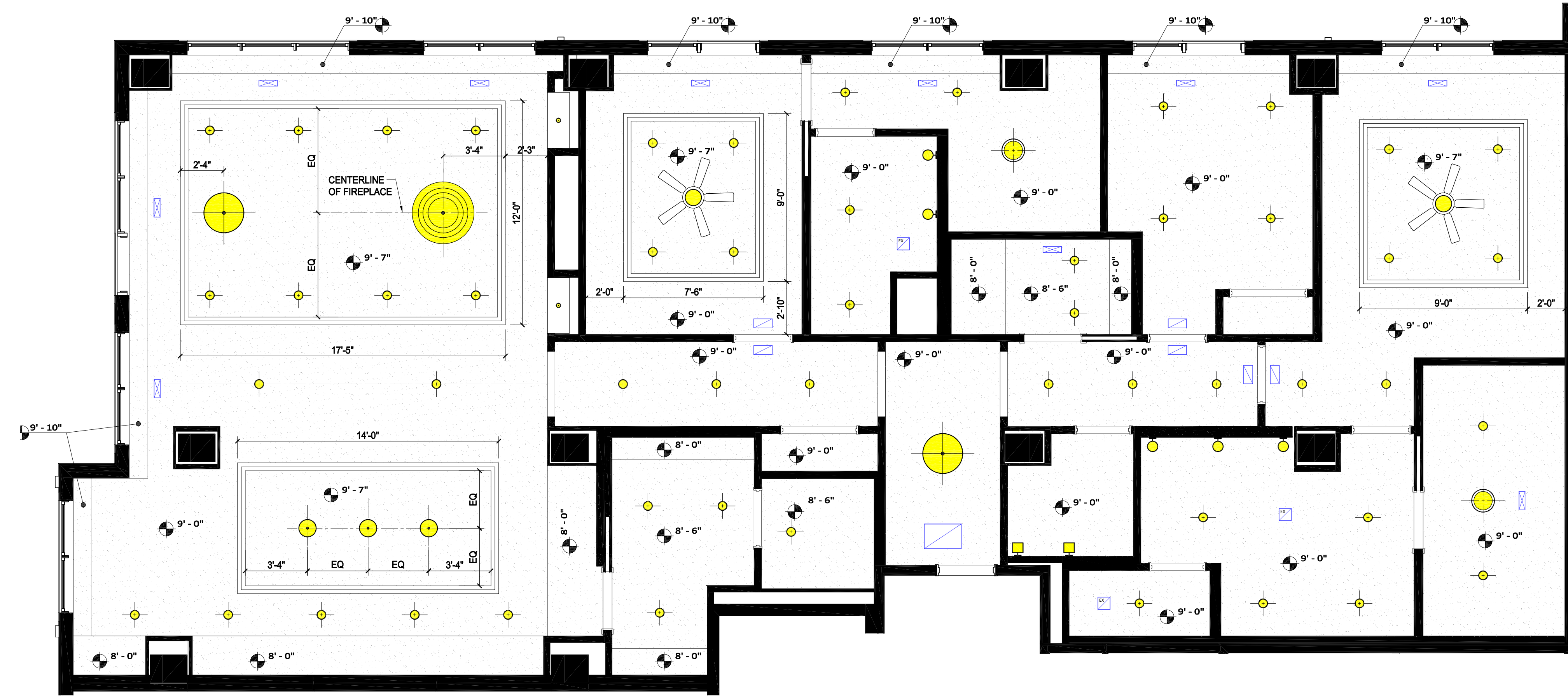
2 CONDO UNIT 302 - REFLECTED CEILING PLAN
