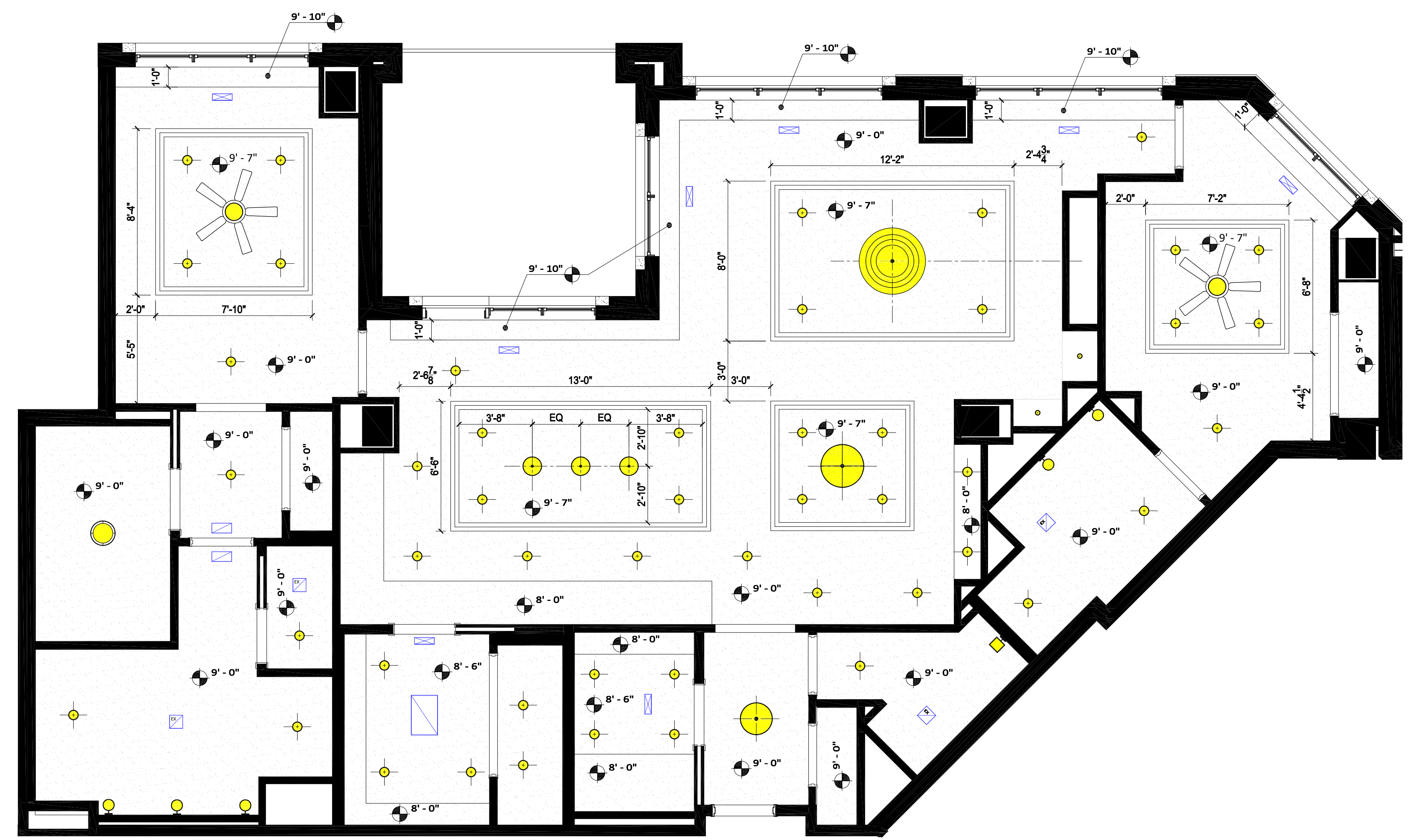
2 CONDO UNIT 208 - REFLECTED CEILING PLAN 1/4" = 1'-0"
